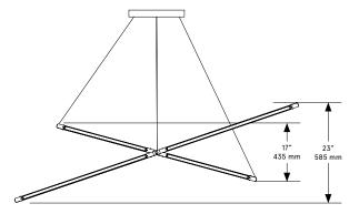
Min. Drop: 34" / 865 mm as shown Angles are adjustable
